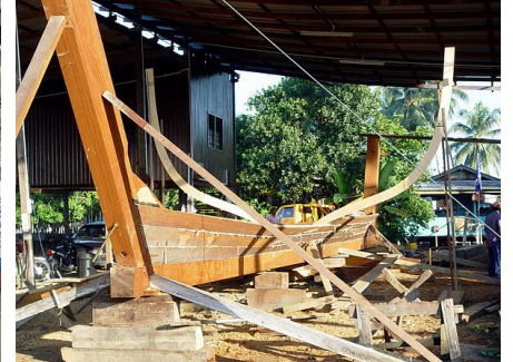
Construction without frames
