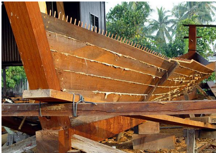
All planks are joined with wooden dowels
