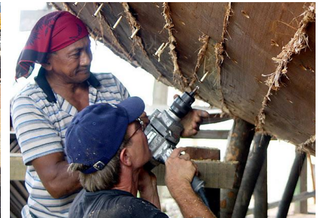
Like all through-hull fasteners these screws are made of silicon bronze
