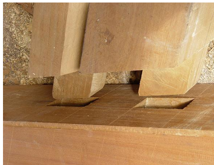
Construction detail, fitting the sternpost
