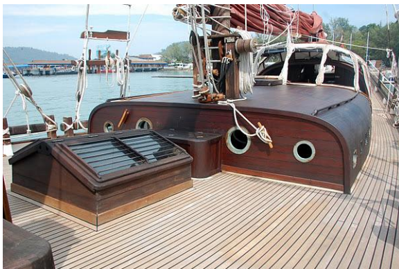
Decks house, skylight and main cabin
